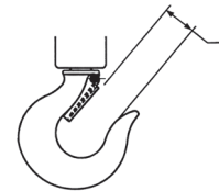
Figure 5 - Inspection du crochet
